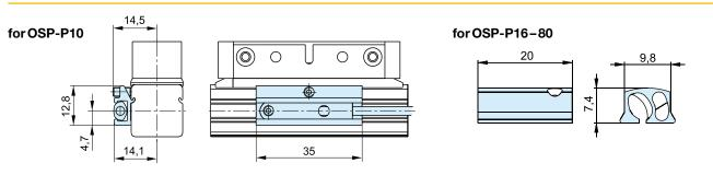
Note for OSP-P10: Switches can not be mounted directly opposite of the carrier !
