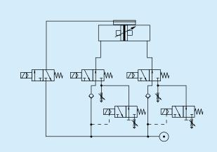
Fast/Slow speed cycle control with pneumatic brake for accurate positioning at high velocities. Additional 3/2-way valves with adjustable throttle valves at the exhaust of the standard directional control valves for two displacement speeds in each direction of the piston's travel. The valve controlling the brake is activated after the slow speed cycle is activated
