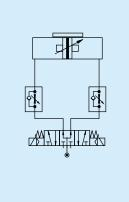
Circuit diagram for end of stroke application. Intermediate positioning is also possible.
