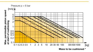
\* For cylinders with linear guides or brakes, please be sure to take the mass of the carriage or the brake housing into account.
