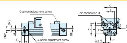
\* Versions of air connection positions 1=>1 or 2=>2, the unused connection must be closed!
