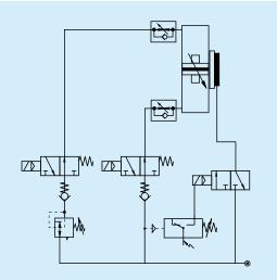
The combination of an OSP-cylinder with the passive MULTIBRAKE as shown here, allows accurate positioning and safety in case of loss of pneumatic air pressure.
