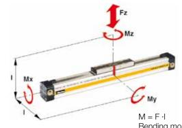
$M = F \cdot I$ Bending moments are calculated from the centre of the linear actuator
